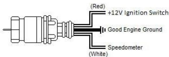
If replacing a cable: screw the provided sender onto the 7/8" male fitting you located previously for the existing electronic sender. If a two-wire sender, you should hook one of the two wires to the speedometer signal wire on the speedometer and the other wire to the ground.
