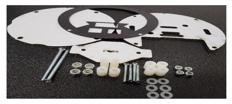
Rear mounting plate: Put the (2) #6 x 2" Recessed Phillips head screws in rear mounting plate. Next, use the (2) #6 x 3/8 Nylon spacers. Next, (2) #6 x 3/4" Nylon spacers then use two of the (4) #6 Nylock nuts. Set 2 Nylock nuts aside you use them to mount Assembly to housing later. Tighten these down because these are going to be mounting points later.
