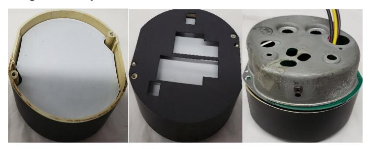
Remove all the old gauges. You may need to do trimming on bezel to make them fit right. The gauge pods Require no additional hardware to assemble. Place lens in bezel then overlay and gauge unit in bezel. Use the factory Bezel and hardware to assemble.
