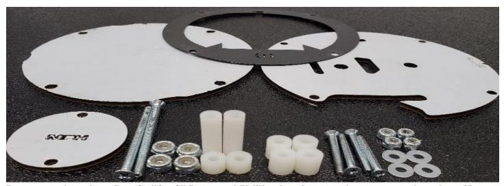
Rear mounting plate: Put (2) #6 x 2" Recessed Phillips head screws in rear mounting plate. Next, (2) #6 x  $\frac{1}{4}$  "Nylon spacers. Next, (2) #6 x 1" Nylon spacers. Next, (4) #6 Nylock nuts. Set 2 Nylock nuts aside you use them to mount Assembly to housing later. Tighten these down because these are going to be mounting points later.
