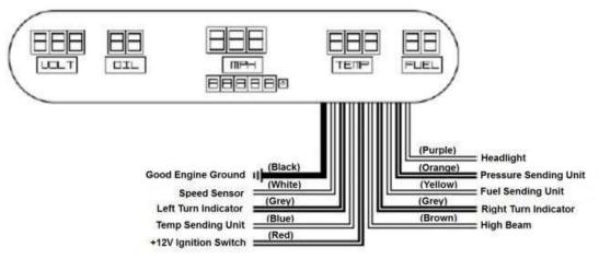
Note: Automotive circuit connectors are the preferred method of connecting wires. You may solder if preferred.
